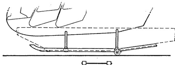
**FIGURE 1-3B FLOAT SHIP GROUND HANDLING WHEELS INSTALLATION**
